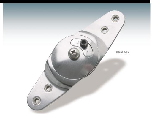
The Camber Axis Hinge® was developed by David J. Hoy, CPO to provide an adjustable ROM ankle joint with anatomical axis alignment for use in thermoplastic orthoses. Equipped with seven different color coded ROM keys (0° stop pictured above), the Camber Axis Hinge® eliminates the need for posterior stop mechanisms. This ankle joint permits solid ankle or variable anterior/posterior stop settings. Manufactured of 410 stainless steel for strength and durability. From Becker Orthopedic.
